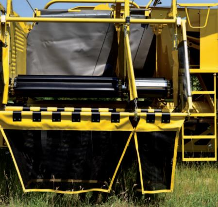
Divided bunker with pad-roll floor for gentle filling. The automatic bunker filling is easier for the driver and ensures the best possible use of the bunker capacity
