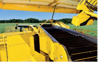
Divided chutes and five steplessly adjustable sorting rollers make it easy to sort undersized items into the separate
