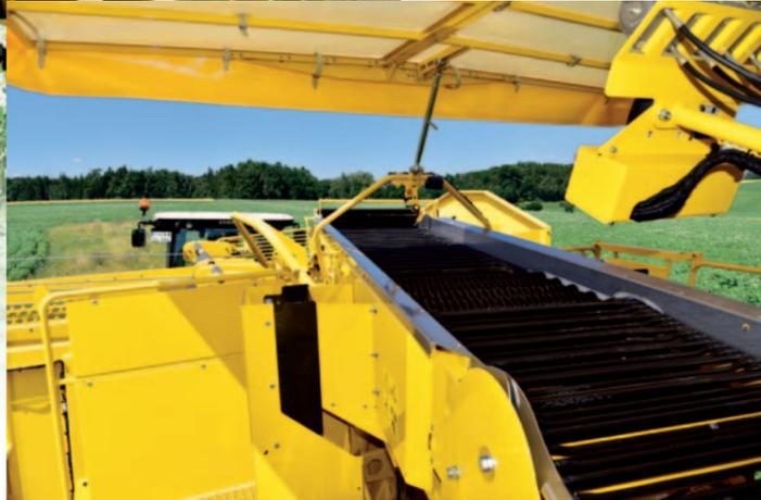
Divided chutes and five steplessly adjustable sorting rollers make it easy to sort undersized items into the separate bunker
