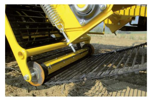
Sieve conveyor tensioner with integrated cleaning roller
