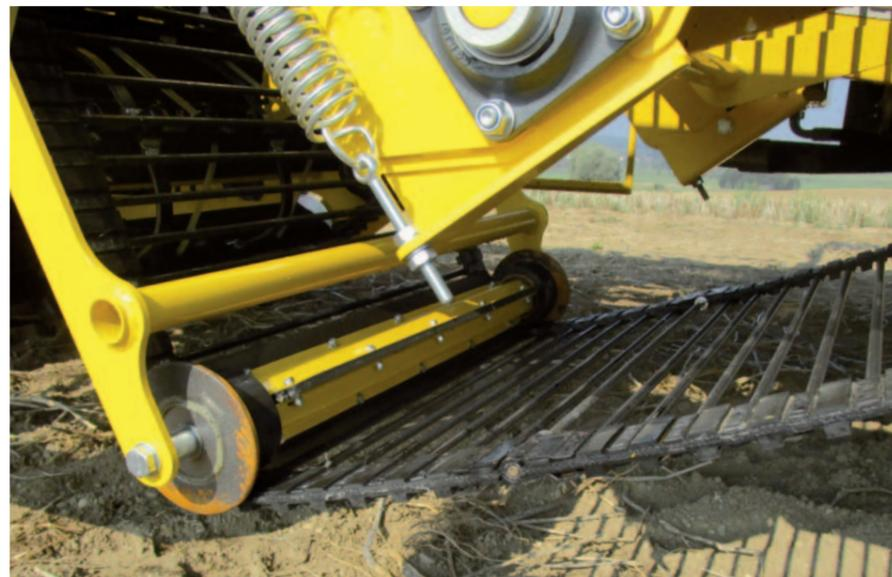
Sieve conveyor tensioner with integrated cleaning roller
