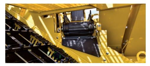
Trash return conveyor on sieve conveyor 2
