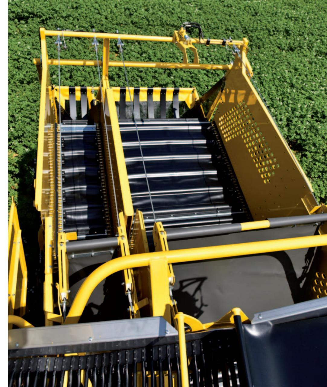
Divided bunker with pad-roll floor for gentle filling. The automatic bunker filling is easier for the driver and ensures the best possible use of the bunker capacity
