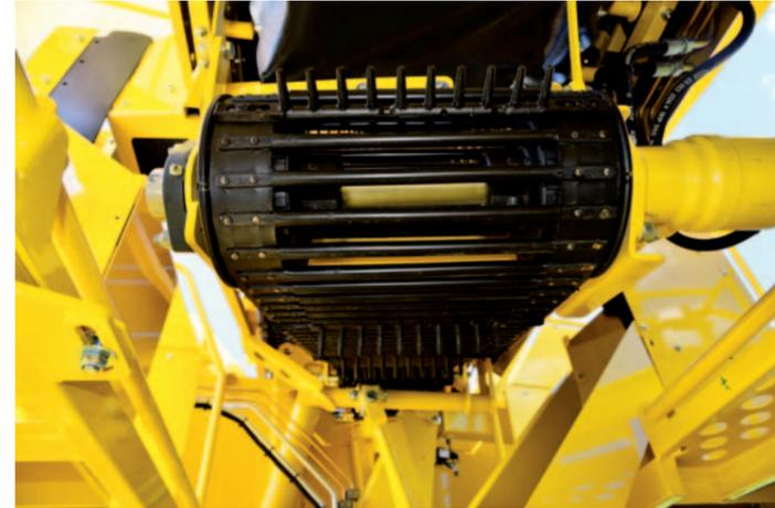
Perfectly integrated feeding conveyor for optimal filling of the separate bunker
