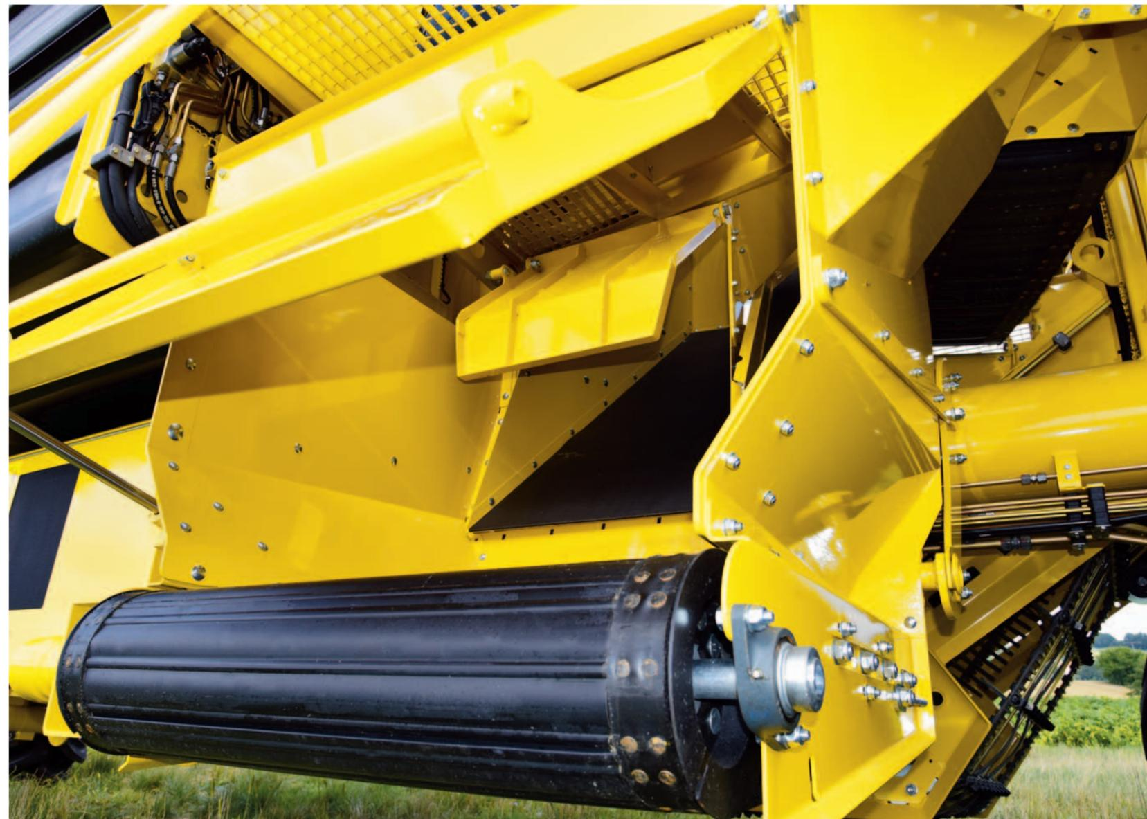
Grader container (internal), can be combined with collection box
