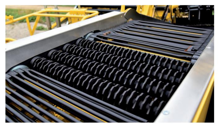
Grader rollers, steplessly adjustable from 25 to 40 mm
