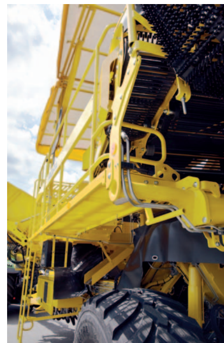
Sorting platform can be swung out for even more space
