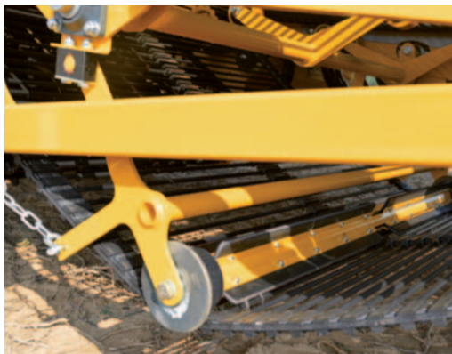
Sieve conveyor tensioner with integrated cleaning roller
