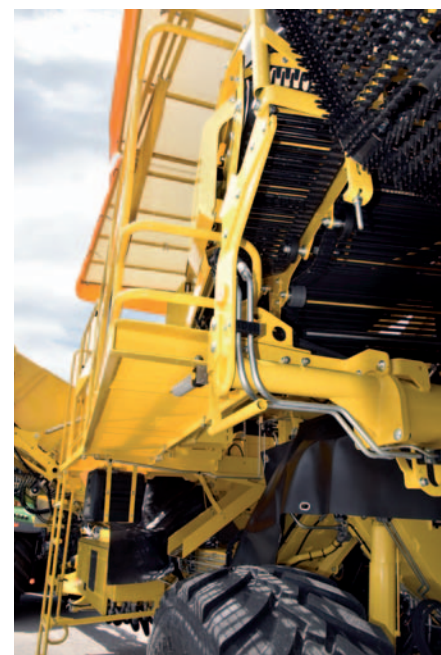
Sorting platform can be swung out for even more space
