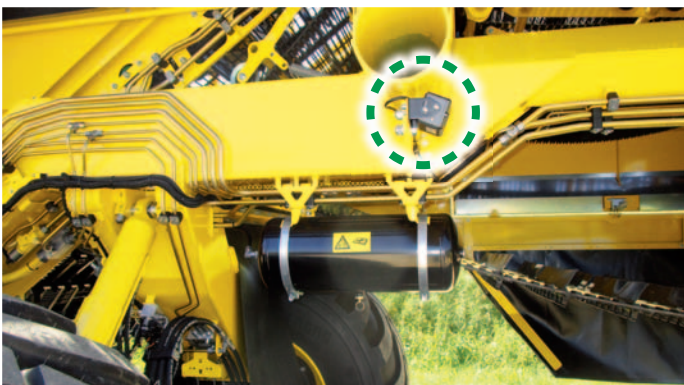
Additional cameras for sieve conveyor, leaf chain, pintle belt, picking table, bunker and reversing
