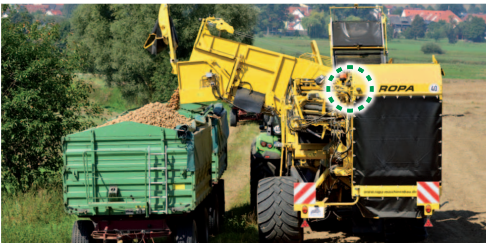
Additional cameras for sieve conveyor, leaf chain, pintle belt, picking table, bunker and reversing
