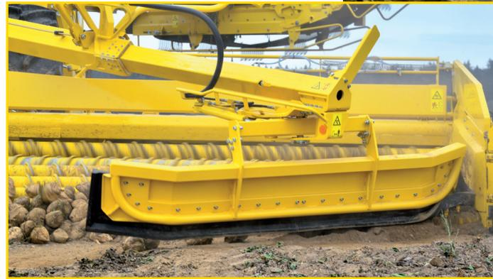
Sturdy residual beet pickup with angled corners, proportionally controlled
