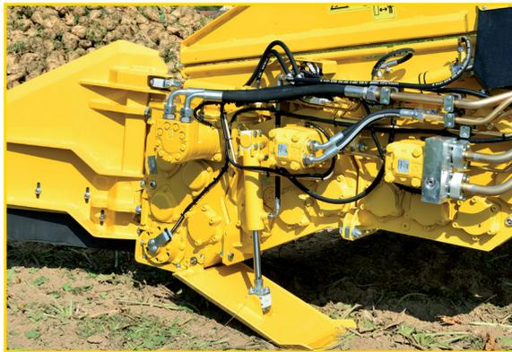
Separate drives for 3 groups of rollers with individual rotational speed adjustment and automatic reversing for stone protection
