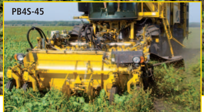
PB4S - defoliator with leaf ejection (4 topper wheels)
