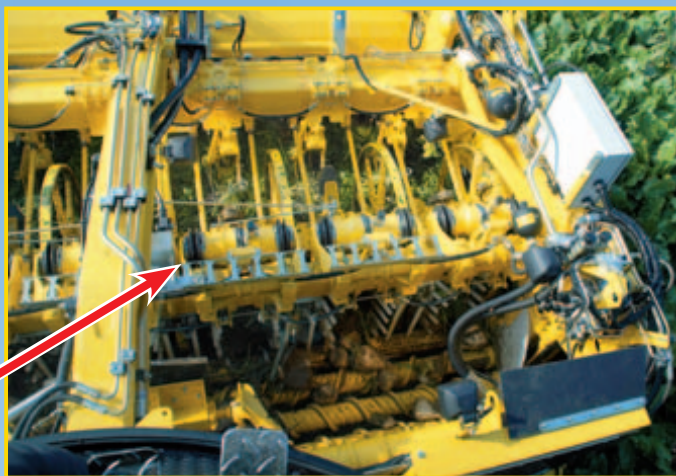
Excellent view across the lifting unit -> the operator watches the beet row and the operation of the Micro-topper
