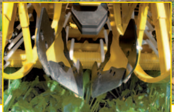
Hydraulic height adjustment of the lifting rollers
