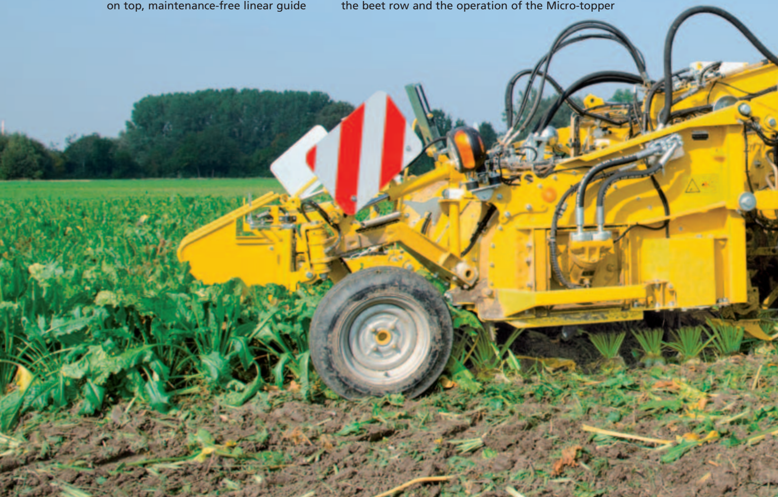
Hydraulic stone protection, positioned on top, maintenance-free linear guide
