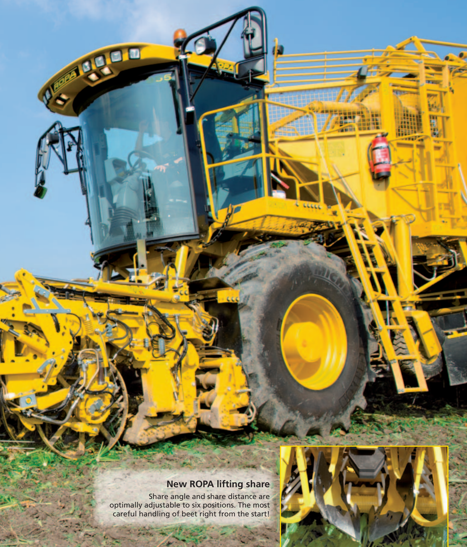
Hydraulic height adjustment of the share shaft
