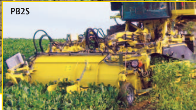
PB2S - defoliator with leaf ejection (2 topper wheels)
