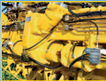
The oscillating shares drive with spur gear and adjustable taper roller bearings.
