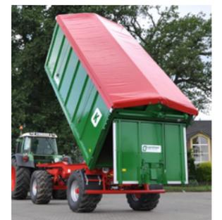
The hydraulic opening side board wall
