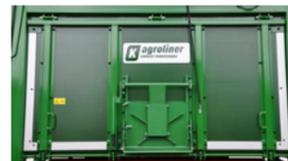
Discharge chute with slide gate. The large slide gate can be easily operated. Max. 1 grain feed can be supplied in the tailgate with the "S" version.
