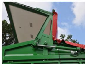
**The hydraulic opening side board wall**
