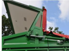
**The hydraulic opening side board wall**
