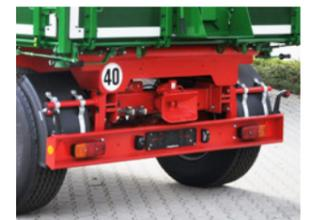
**Underride protection and the towing hitch**
