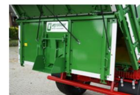
**The portal function** As the first in the industry, we provide our customers with a board wall portal function for easy loading of pallets or other bulky goods (available for the rear and also the side board walls). Naturally, the swivel function of the board walls remains. Handling is safer and even more user-friendly.
