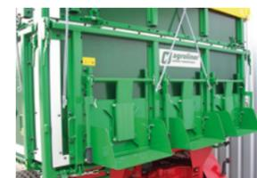
**The split board wall** give more ground clearance when tipping and reduce the load's surge pressure.
