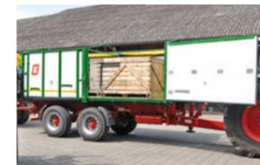
**The overhead loading side panels** To effectively reduce the height potatoes fall when being overhead loaded, we have developed a special side panel system. They are secured using two long-lever locks and can be easily and quickly folded up and locked using a hand-pump or the tractor unit's hydraulics.
