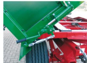
**Smart Lock** With our patented hydraulic board wall locking system, the side tipping process can be handled completely from the tractor cab. With the purely mechanical alternative solution, the centre locks for horizontal undivided board walls are automatically locked or unlocked, respectively. This provides gains in safety, time, and comfort.
