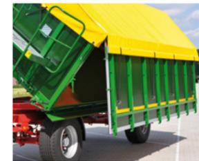
**The discharge chute with slide gate** The large slide gates can be easily operated. As an option, up to three slide gates can be supplied.
