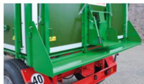
**The Remote unlocking** allows for the lower locking device to be opened from the tractor cab.
