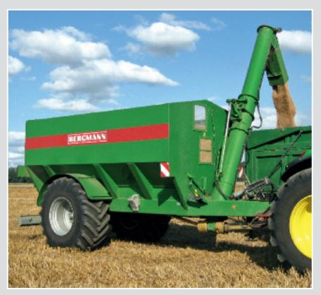
The GTW 21 and the GTW 25 have a 21 m³ capacity. With the optional sidewall extensions 25 m³ can be transported and transferred. A special horizontal feeder conveyor located in the bin moves the harvested material quickly, evenly and carefully into the transfer conveyor.
