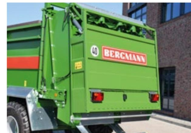
Hydraulically operated **spreader unit hood**.
