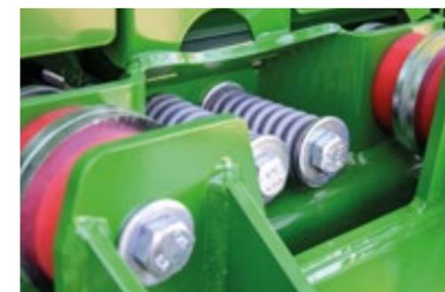
The use of spacers makes it possible to ideally adjust the drawbar height for every tractor. The spring elements provide for high driving comfort.
