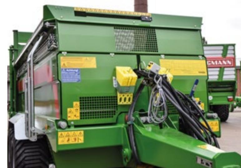
Exact height indicator for the optional hydraulic dosing wall. The protective screen provides for a good view of the scraper floor chains. The cargo space and transport floor can be seen easily through the window.
