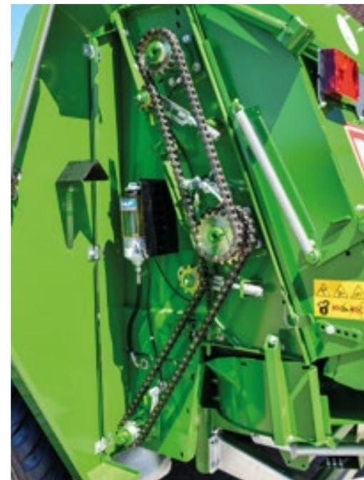
**TSW spreader unit drive** via roller chain. Spring-mounted chain tensioners ensure optimum power transmission and low wear.
