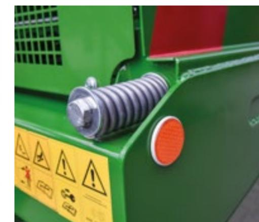
With the automatic tensioning system, which is visible from the tractor, the four high-strength scraper floor chains can be easily adjusted from the front. This allows for a high degree of safety and smooth operation.
