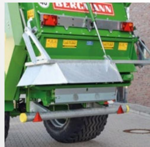
The optional, hydraulically operated **spread pattern limiter** prevents the contamination of roads, paths and waterways etc. and ensures precise and uniform spreading of fields, right up to the edges.
