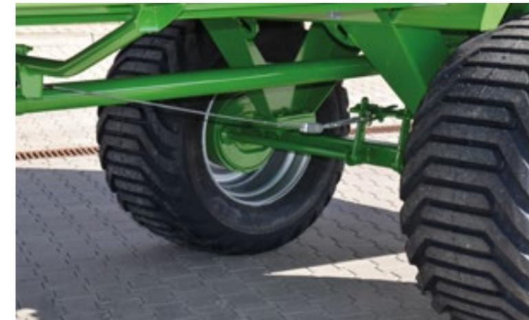
Wide tires with low tire pressure prevent soil compaction.
