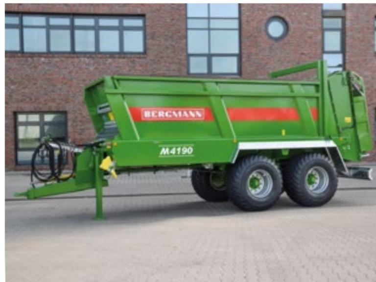
**Optional high or low drawbar** with spring-mounted drawbar for high driving comfort and good driving stability. The use of spacers makes it possible to ideally adjust the **drawbar height** for every tractor.
