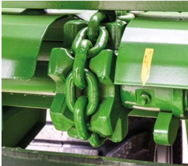
The hydraulic **scraper floor drive** ensures transport of the most diverse materials to the spreader unit.
