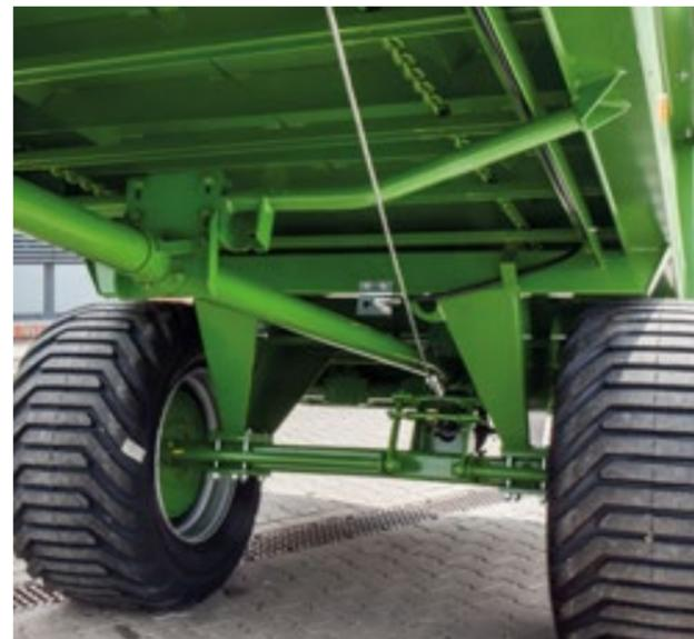
The **self supporting bin** eliminates the need for a supporting frame and thus offers almost no possibilities for dirt to collect. Both result in minimum maintenance and cleaning times.
