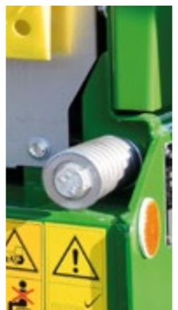
The use of spacers makes it possible to ideally adjust the **drawbar height** for every tractor. The spring elements provide for high driving comfort.
