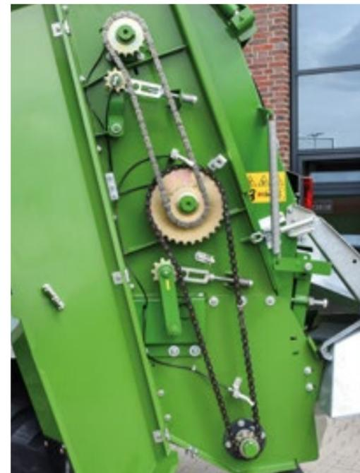
**TSW spreader unit drive** via roller chain. Spring-mounted chain tensioners ensure optimum power transmission and low wear (left). The optional **cardanic drive** minimizes maintenance and provides high power reserves. The M SZ spreader unit is driven via PTO shaft and chainless drive train.
