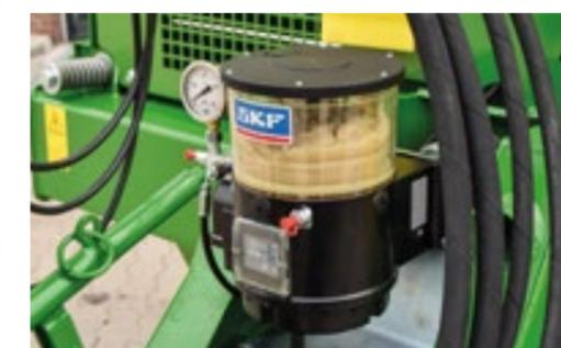
The optional central lubricating system provides for a continuous flow of lubricant which is adapted for each individual bearing. This significantly reduces maintenance efforts.
