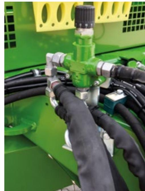
The optional **manual scraper floor control** makes exact material dosing possible.
