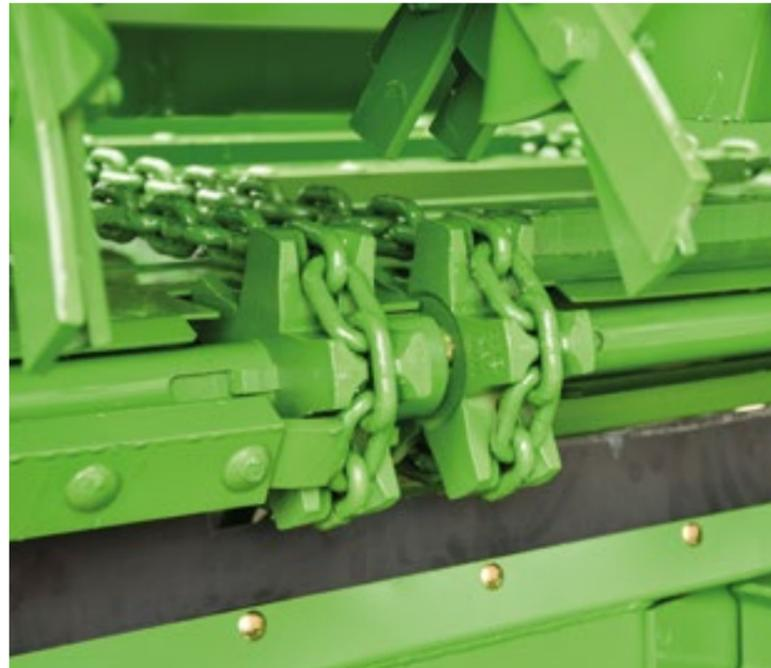
The hydraulic **scraper floor drive** with spur gear box ensures safe transport of the most diverse materials to the spreader unit. A reinforced drive is optionally available.
