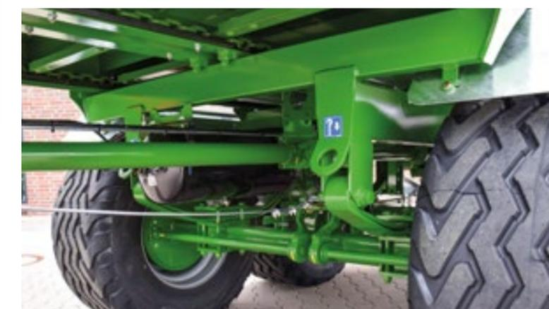
Standard overrun brake with auto-reverse. Air brakes and hydraulic brakes (without ALB) are optional.
