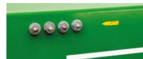
All lubrication points are easily accessible or grouped into lubrication blocks for quick and easy maintenance.
