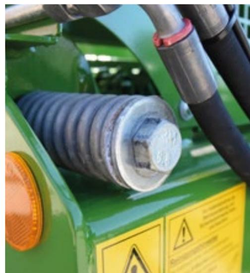
The automatic **scraper floor chain tensioners** are mounted on the front side of the trailer and are visible from the tractor. They can be easily adjusted from the outside.
