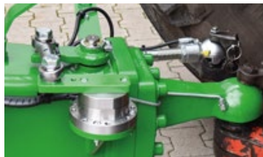
Forced steering (hydraulic or computer controlled) is optionally available. The computer-controlled forced steering is equipped with emergency features.
