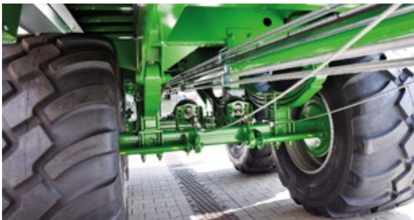
BERGMANN TSW 5210 W (W = Weighing) The TSW 5210 W as standard with a weighing system with high-resolution weighing bars for high precision.
